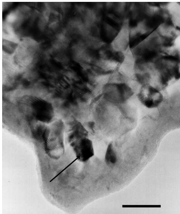
Fig. 8. TEM observation of kaolinite transformed phase, fired at 1050 °C, indicating the presence of iron rich clusters. Bar = 100 nm.
